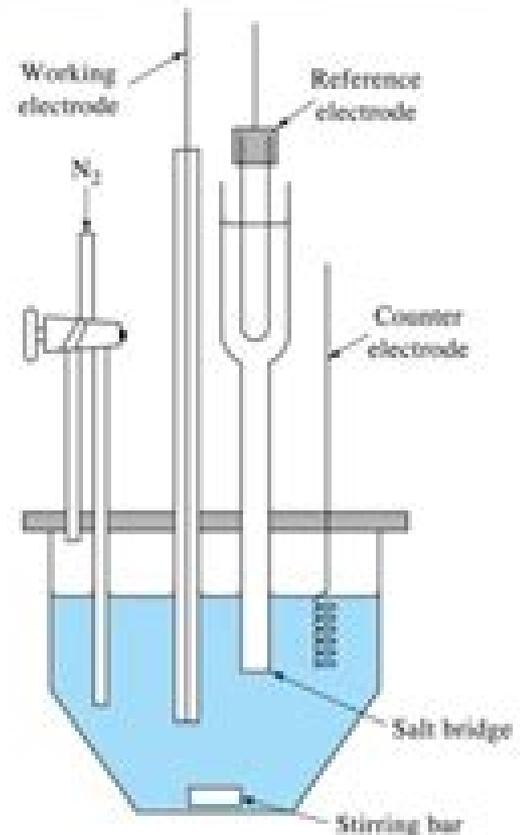
Fig. 25-8 (p.724) A three-electrode cell for hydrodynamic voltammetry.
