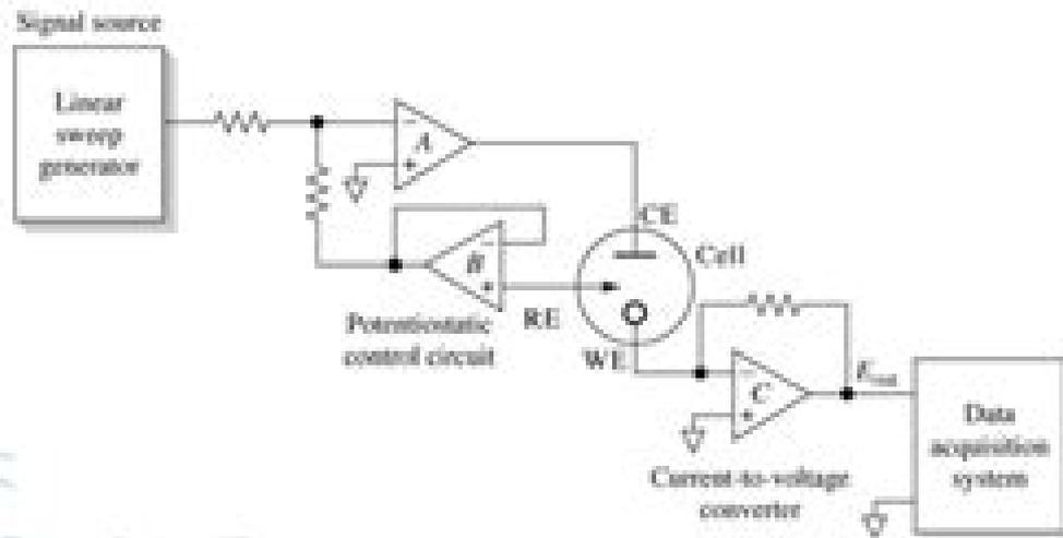
Fig. 25-2 (p.718) A system for potentiostatic three-electrode linear-scan voltammetry
